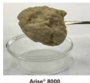
Figure 5. Appearance of hydrated Arise® 8000 showing its elastic properties (1 part Arise® 8000 to 2 parts water).
